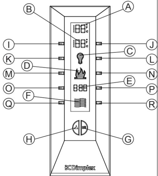
button. Set the timer from 30 minutes through 8 hours. The fireplace will automatically turn off when the sleep timer reaches zero (0) minutes.
