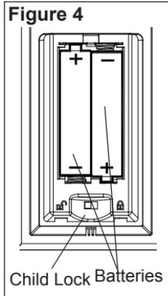
1. Depress the tab on the battery cover on the back of the remote control and remove battery cover.
