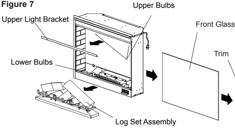
the Log Set contains LED's and wires.
